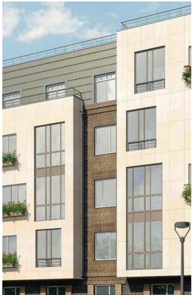
3.14-1: Brick, stucco and metal shingles are materials common to an eclectic “Main Street” like Bloomfield Avenue. They can be combined in forms that resonant with the old while feeling fresh and new.
