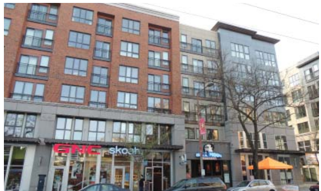
1.3-3: Discouraged: The base-middle-top facade strategy is rooted in traditional design, as are varied setbacks and cornices. When the materials and details of local design examples are ignored, however, new buildings can appear generic and cookie-cutter.
