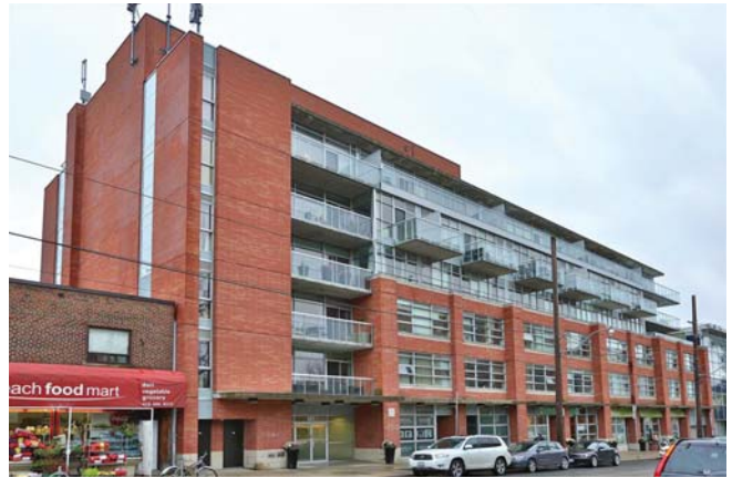
3.4-18: A three-story brick and storefront base (right) ties into the existing, lower context while a vertical brick mass (left) announces the transition to a taller re-zoned area. Stepbacks from right to left and glass "infill" zones mitigate overall mass.
